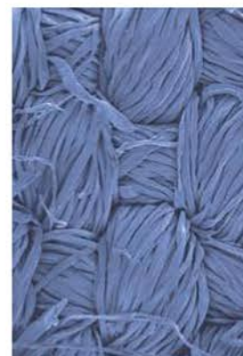
Scanned electron microscopy image of the graphene-cotton fabric.
