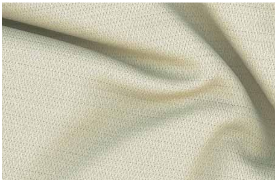
Double mesh fabric from Deer Creek, knitted with Sorbtek, Reflexx, and X-Static. The outer layer is Sorbtek and the inner layer is Reflexx for stretch and recovery.
