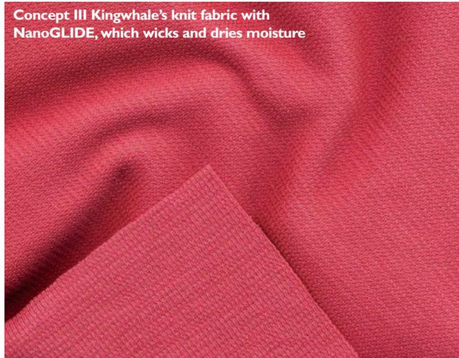
abrasion that can cause wear and damage to the garment surface. According to Concept III, NanoGLIDE is more than nine times more abrasion resistant than performance nylon and polyester without the technology. NanoGLIDE protection is washable and also addresses UV degradation by providing more tensile strength after UV exposure.
