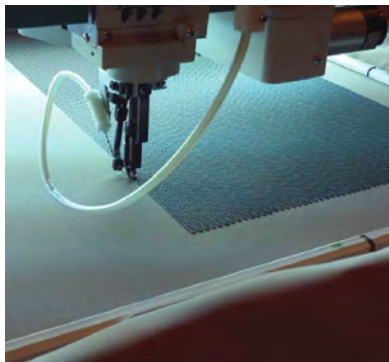
Tajima's TLMX series Heater Wire Sewing Machine, sewing heater-wire onto a fabric
