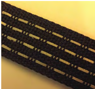
American Cord & Webbing's 3M reflective tape woven into a Kevlar webbing
